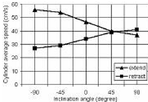
Fig.5. Effect of inclination angle to cylinder average speed with load of 5 kg
