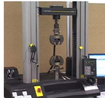
Gambar 3. Ultimate tensile machine(UTM) servo-hydraulic INSTRON
