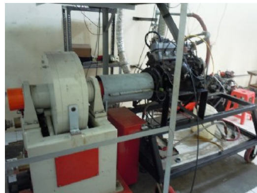
Gambar 1. Engine Test Bed Dynamite dan motor bakar bensin (Otto)
