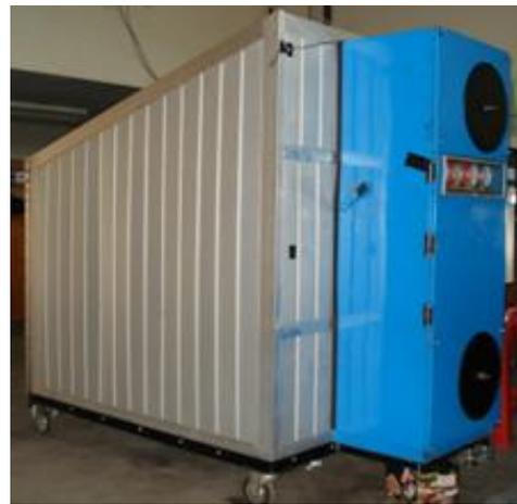
Gambar 4. Alat pengering *thermal collector - heat pump*.
