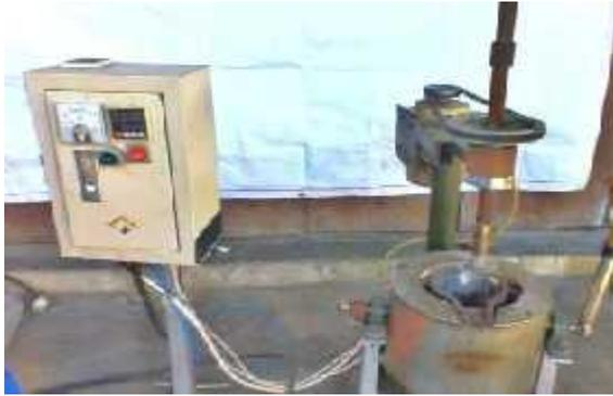
Gambar 2.1. Tungku *Stir casting*
