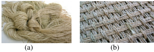
Gambar 2. (a) Serat cantula pilin (b) Anyaman 3D.
