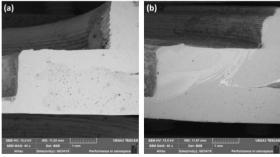
Figure 6. SEM test results: (a) Variations without Zn interlayer; (b) Variations with the Zn interlayer
