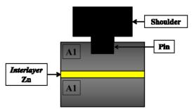
Figure 3. Zn interlayer placement scheme
