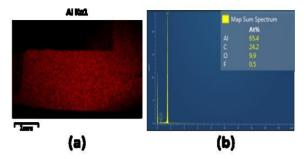
Figure 7. (a). Mapping test results on specimens without Zn interlayer; (b). EDS test results on specimens without Zn interlayer.
