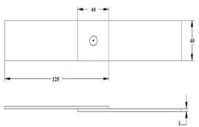
Figure 2. FSSW specimen size scheme
