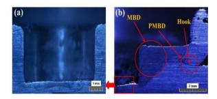
Figure 5. Material Flow in Regions (a). Under Keyhole; (b). MBD and Hook Defect
