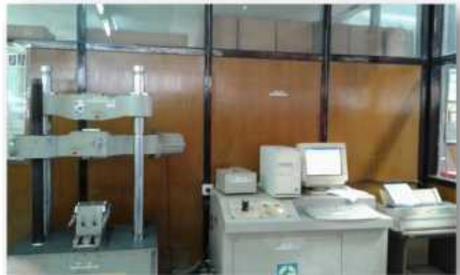
Gambar 7. GOTECH Universal Testing Machine
