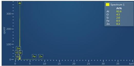
Figure 4.10 EDS testing result on 70 A, 10 L/min
